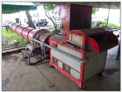
This mechanical dryer is used for higher volumes of palay. Some models operate on rice hull. Only some millers and FOs own a flatbed dryer.
