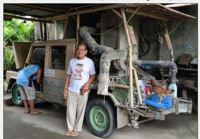
Mobile milling facilities only handle small volumes of palay. The palay undergoes only one polishing step, thus producing milled rice of low quality. In most cases it is intended for self-consumption purposes.
